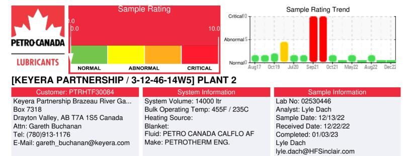
Recommendation: Units are being sampled at very short intervals recommended sampling for heat transfer systems with no issues is 12 months. Sample results indicate that the fluid is in suitable condition for continued service.
