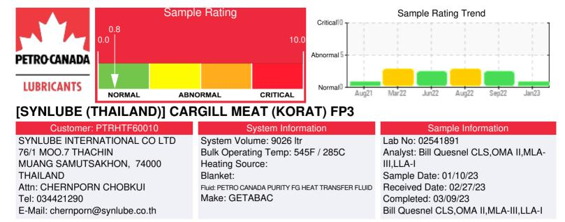
Recommendation: The flash point has been restored. If you were venting the expansion tank, continue to do so every month to reduce the amount of light ends present in the thermal fluid. The fluid is suitable for further service. Resample at the next service interval to monitor.
