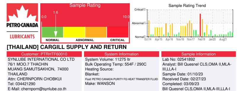
Recommendation: With exception of the COC Flash Point that is marginally low, all other parameters remain within acceptable limits. Please re-sample at normal frequency, oil if fit for further use
