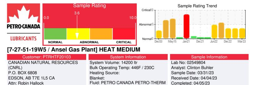
Recommendation: Fluid degradation continues to progress. Fluid viscosity, Acid Number, solids and iron content all have increased since the sample taken on December 31, 2022. The system requires cleaning, flushing and refill with fresh heat transfer fluid.
