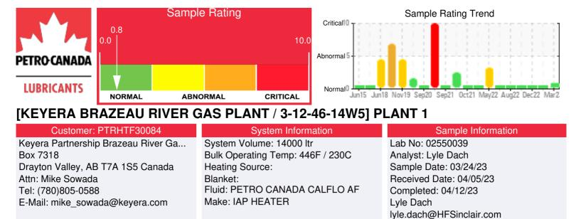
Recommendation: Sample results indicate that the fluid is in very good condition and would be suitable for continued service. Water content is very low, 10% distillation of 385°C would be considered within spec of new fluid. Resample in 12 months.
