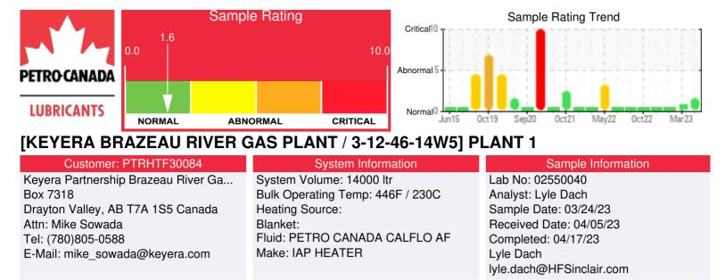
Recommendation: Fluid is in good condition overall. Sulfur, viscosity, 10% and 90% distillation are slightly high. Sample location could have affected the results, this sample was collected from the seal flush tank. Water content is low.
