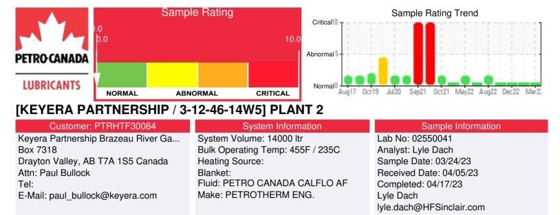
Recommendation: From the sample results fluid condition is very good, the sample color looks similar to the last sample collected on March 4 2023. This sample was collected from the seal pot. Water content is very low.
