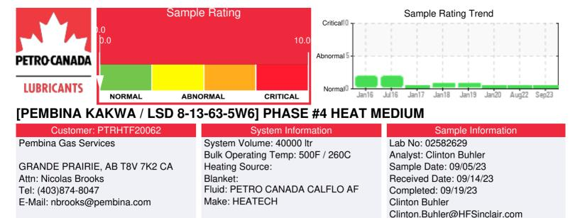
Recommendation: Sample results indicate the fluid is in suitable condition for continued service. Iron concentration has increased slightly, yet the fluid's Acid Number remains low.Please re-sample in 12 months.
