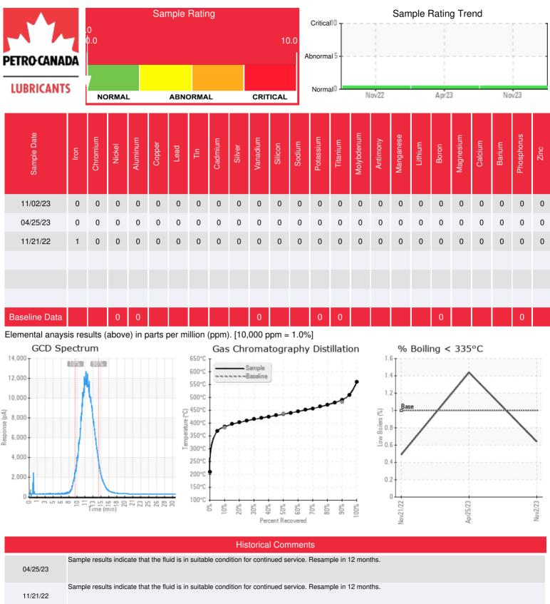
Sample results indicate that the fluid is in suitable condition for continued service. Resample in 12 months.
