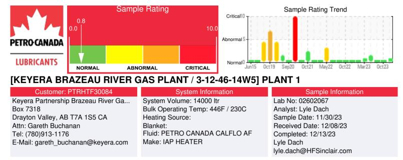
Recommendation: Sample results indicate that the fluid is in suitable condition for continued service. 90% distillation point is slightly elevated, confirm blanket gas is functioning properly as fluid oxidizing could cause the increase. Resample in 12 months.
