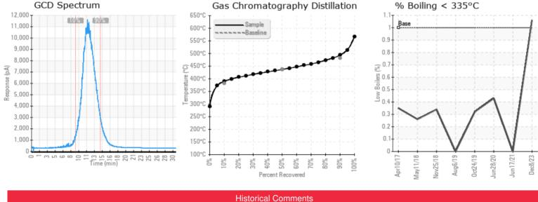
\*\*\*\* sample was 100% water in the metal can. No thermal fluid \*\*\*Please re-sample immediately but ensure that the sample is taken from a representative point; pump discharge is ideal. Please thoroughly purge out sample point until hot heating fluid is coming out before taking the sample. Investigate the source of water contamination. Water contamination levels are severe.
