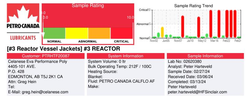
Recommendation: After 9 months of service the fluid is in an excellent condition. Significant improvement has been made compared with the previous fluid fill which was severely degraded in 4 months. Please re-sample in 12 months.
