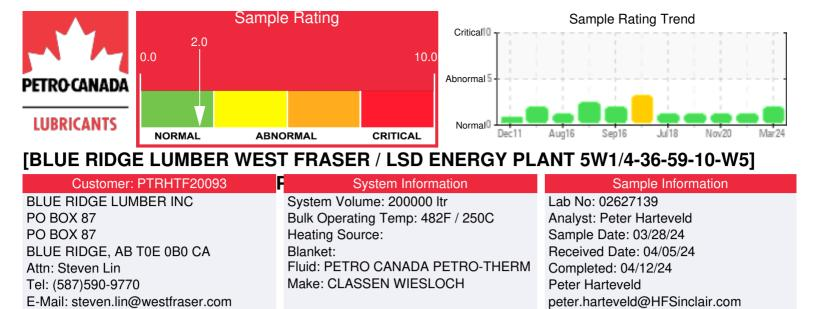
Recommendation: The fluid is in a good condition and suitable for use. The AN is elevated and the 90% GCD temperature is high. These are indications of fluid degradation via oxidation. The Fe content is low which means there is no corrosion ongoing as a result of acidity increase from oxidation. It is recommended to check proper operation of the blanket gas system and keep the fluid temperature in the expansion tank low. Please re-sample in 12 months.
