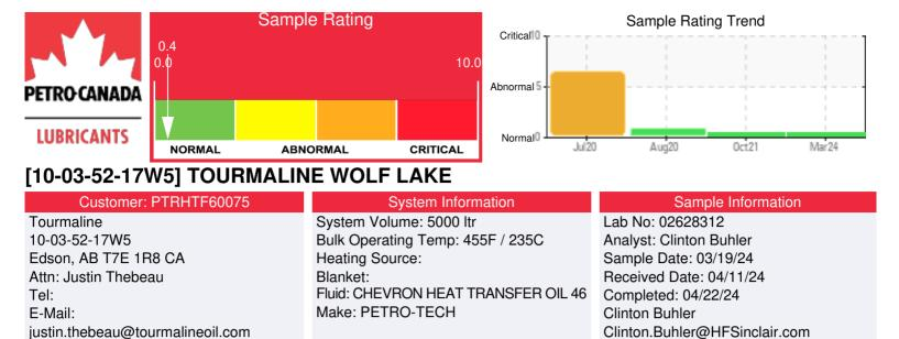
Recommendation: Sample results indicate the fluid is in suitable condition for continued service. Low boiler vapor content has increased to 5.75%; expansion tank venting is helpful in reducing this. Please re-sample in 12 months.
