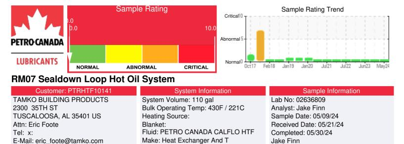
Recommendation: Results indicate that the fluid is in great condition and suitable for continued use. No signs of wear particles, contamination or fluid degradation are present. Continue with regular monitoring at next sample interval.
