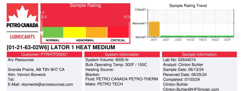
Recommendation: Sample results indicate the mix of Chevron 46 and Petro-Therm is in suitable condition for continued service. Please re-sample in 12 months.
