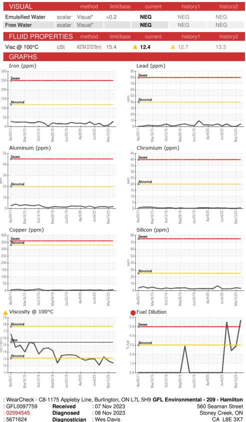
Accredited Laboratory Test Package : MOB 1 (Additional Tests: FuelDilution, PercentFuel) To discuss this sample report, contact Customer Service at 1-800-268-2131. Test denoted (\*) outside scope of accreditation, (m) method modified, (e) tested at external lab. Validity of results and interpretation are based on the sample and information as supplied.
