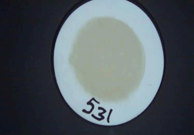
MPC (Varnish Test)
