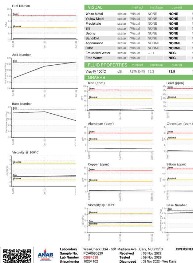
Test Package : MOB 2 (Additional Tests: FuelDilution, PercentFuel)
