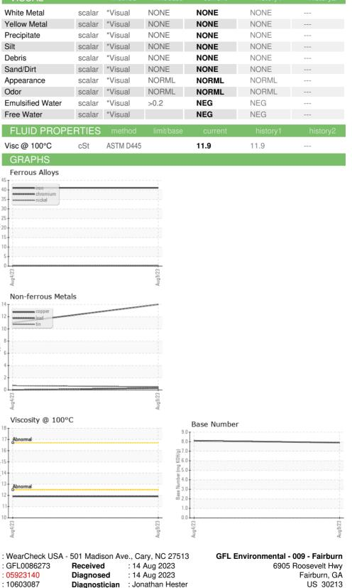
Test Package : FLEET (Additional Tests: FuelDilution) Certificate L2367 To discuss this sample report, contact Customer Service at 1-800-237-1369. \* - Denotes test methods that are outside of the ISO 17025 scope of accreditation. Statements of conformity to specifications are based on the simple acceptance decision rule (JCGM 106:2012)
