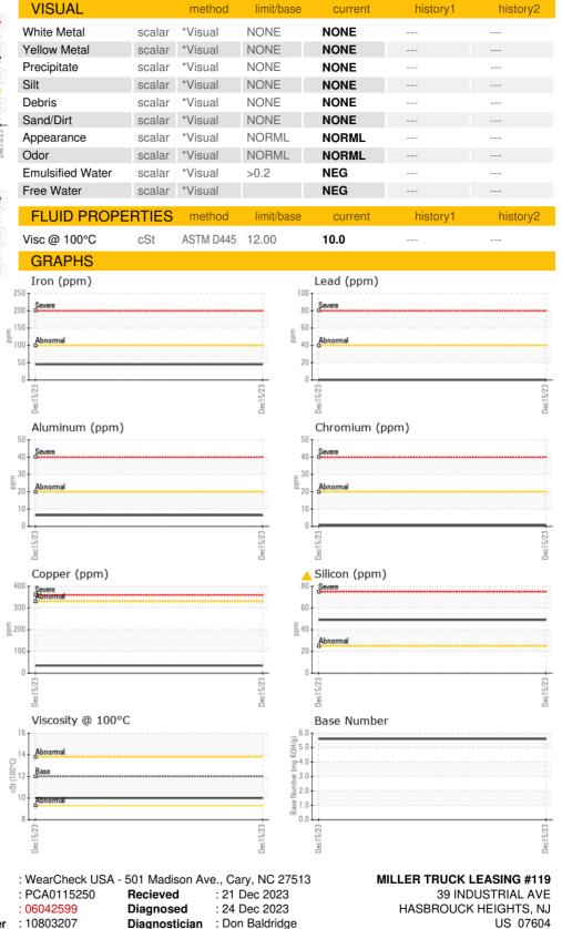
Test Package : MOB 1 (Additional Tests: TBN) Certificate L2367 mlongette@millertransgroup.com To discuss this sample report, contact Customer Service at 1-800-237-1369. \* - Denotes test methods that are outside of the ISO 17025 scope of accreditation. Statements of conformity to specifications are based on the simple acceptance decision rule (JCGM 106:2012)
