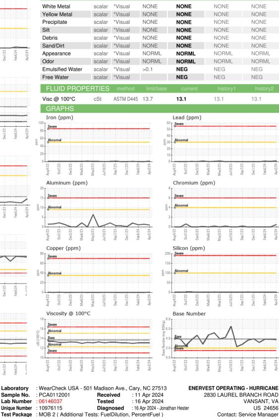
Test Package : MOB 2 (Additional Tests: FuelDilution, PercentFuel) Certificate 12367
