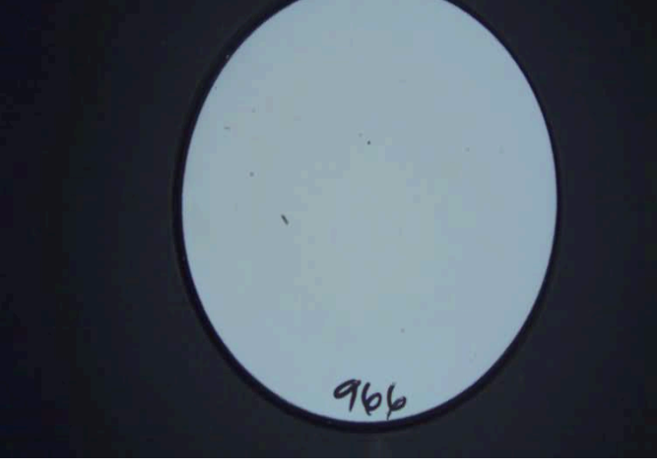
MPC (Varnish Test)
