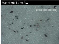
The filter contained no appreciable wear particles. All filter wear levels are normal.
