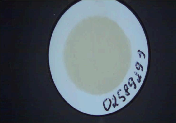
MPC (Varnish Test)
