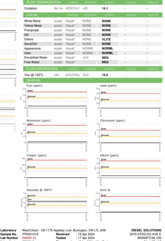
ISO 17025:2017 Accredited Unique Number : 5762246 Diagnosed : 17 Apr 2024 - Wes Davis Laboratory Test Package : MOB 1 (Additional Tests: FuelDilution, PercentFuel, Visual) To discuss this sample report, contact Customer Service at 1-800-268-2131. Test denoted (\*) outside scope of accreditation, (m) method modified, (e) tested at external lab. Validity of results and interpretation are based on the sample and information as supplied.
