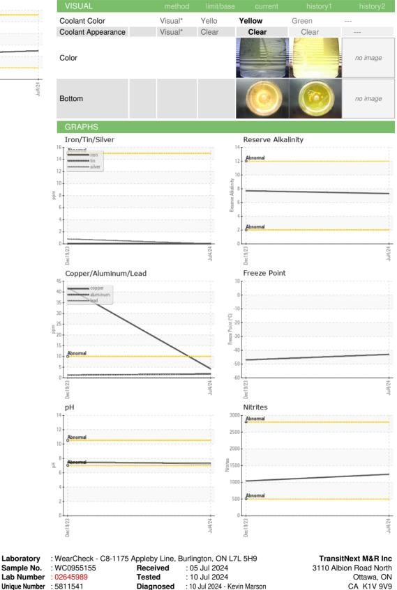
Unique Number : 5811541 Test Package : COOL ( Additional Tests: GlycolType ) To discuss this sample report, contact Customer Service at 1-800-268-2131. Test denoted (\*) outside scope of accreditation, (m) method modified, (e) tested at external lab. Validity of results and interpretation are based on the sample and information as supplied.
