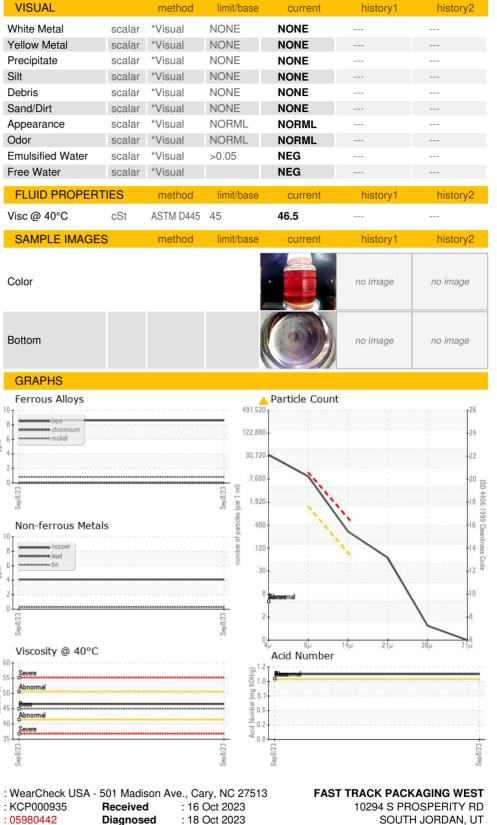
Test Package : IND 2 (Additional Tests: KF, PrtCount) Certificate L2367 To discuss this sample report, contact Customer Service at 1-800-237-1369.
