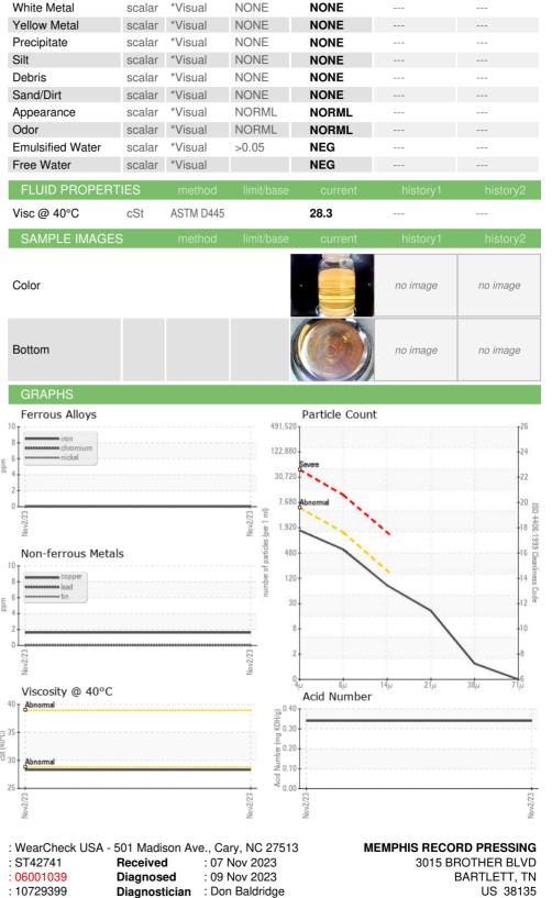
Ab n mac Viscosity @ 40°C 40 Abnorma 38 36 () 00 04 <del>ني</del> 32 30 28 26 Nov2/23 Particle Trend 6 î <sup>5</sup> (40°C) in al . 쟝 30 10 21 0 Laboratory Sample No. Lab Number Unique Number
