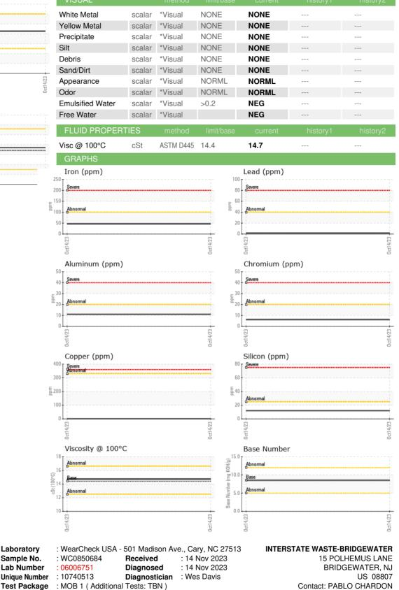
Test Package : MOB 1 (Additional Tests: TBN) Certificate L2367 To discuss this sample report, contact Customer Service at 1-800-237-1369. PChardon@interstatewaste.com \* - Denotes test methods that are outside of the ISO 17025 scope of accreditation. Statements of conformity to specifications are based on the simple acceptance decision rule (JCGM 106:2012)
