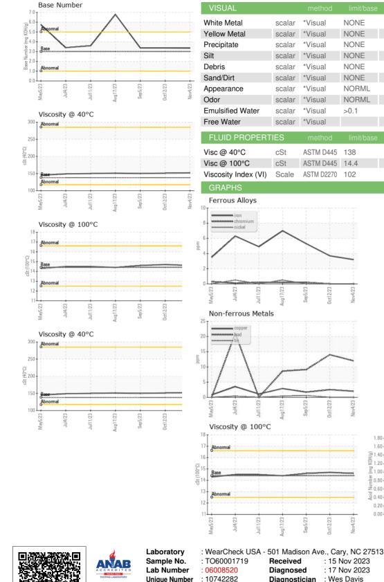
Test Package : IND 2 (Additional Tests: FT-IR, KV40, VI)
