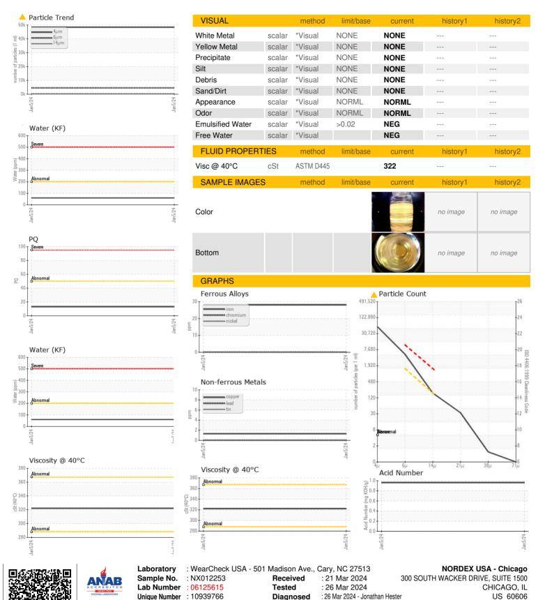
Test Package : IND 2 ( Additional Tests: KF, PQ, PrtCount )
