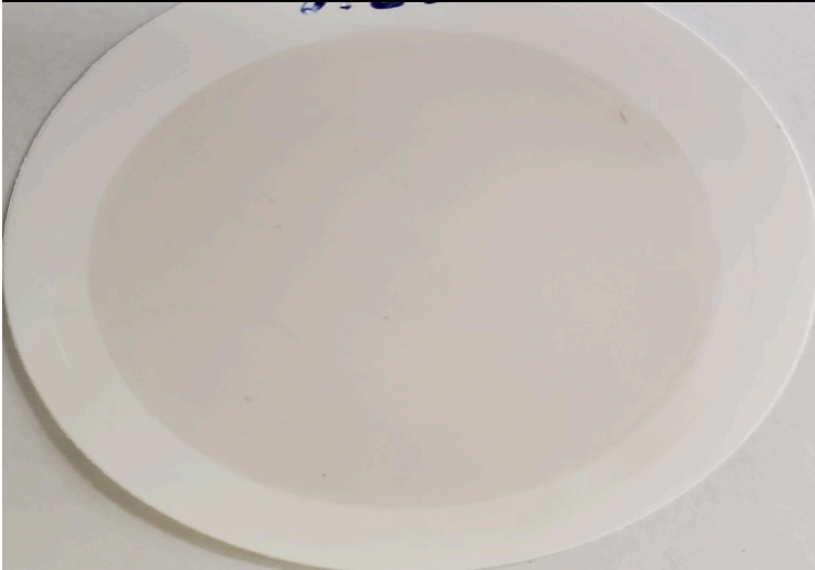
MPC (Varnish Test)
