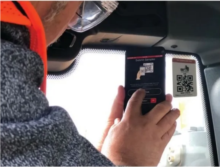
Asset tags provide a simple and reliable way of correctly identifying sample points for oil analysis every time a sample is taken.
