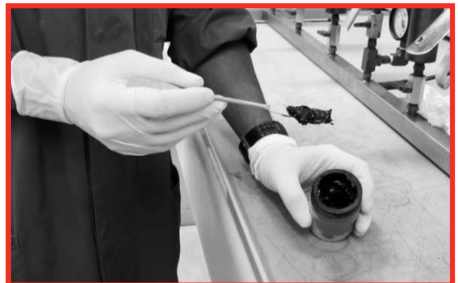
Heavily sludged engine oil (soot contamination)
