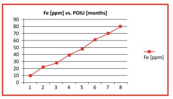
Figure 8: Normal wear profile for components with many samples between drains
