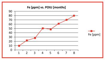
Figure 9: Increased wear at sample 4
