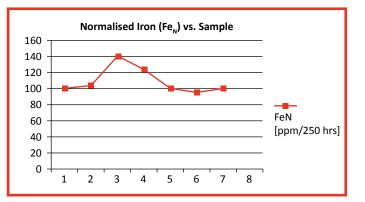
Figure 7: Normalised wear readings versus sample
