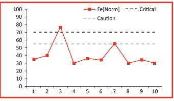
Figure 11: Normalised wear readings with calculated statistical limits superimposed
