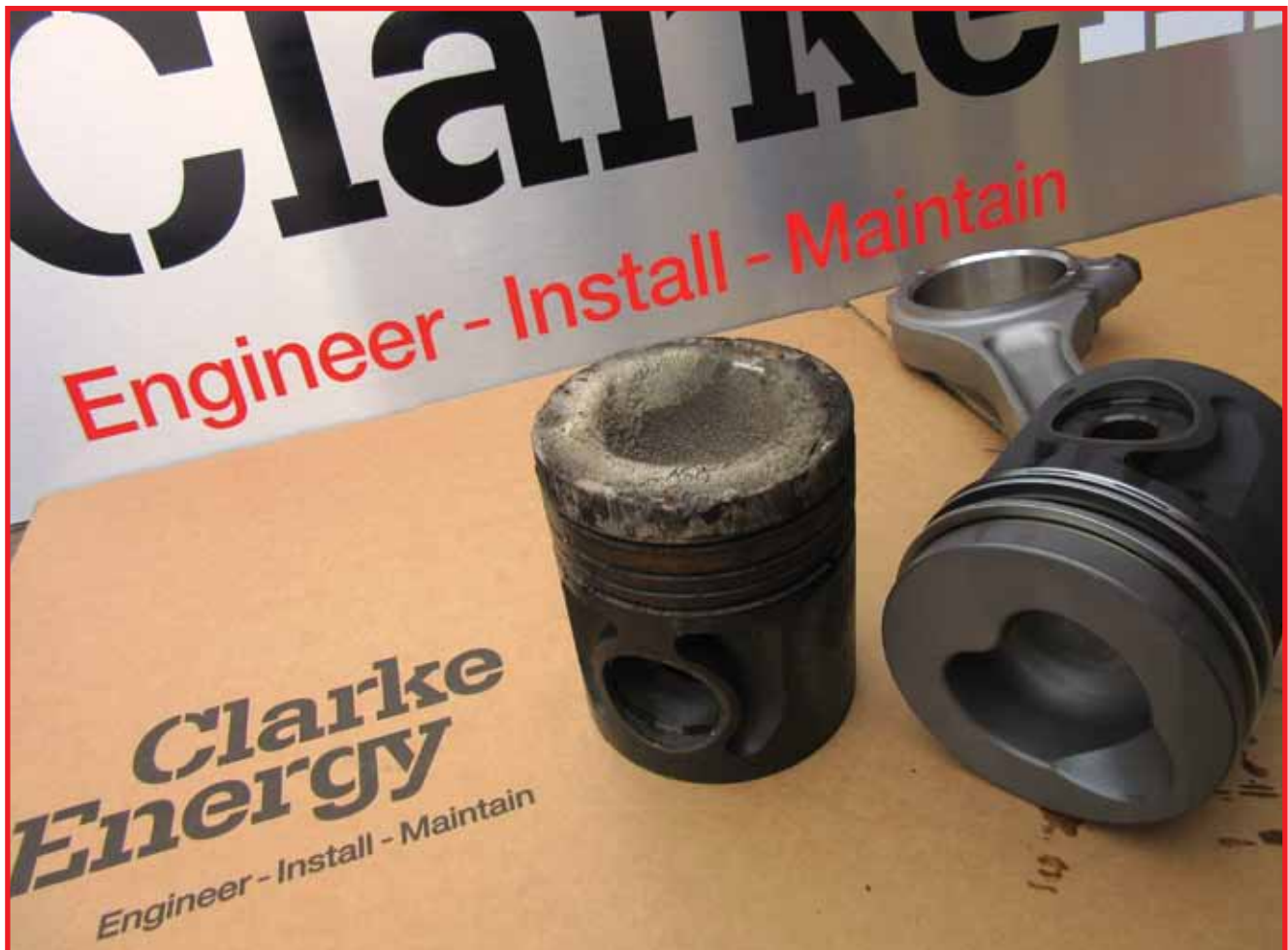
New and siloxane coated piston courtesy of Clark Energy
